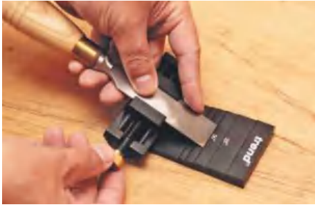
▲ You slide the blade through until it rests against the ridge of the required hone angle
